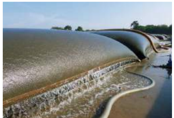
Food processing wastewater ➤ After coagulant added ➤ Followed by flocculant added ➤ Clear effluent
