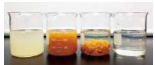
Food processing wastewater ➤ After coagulant added ➤ Followed by flocculant added ➤ Clear effluent
